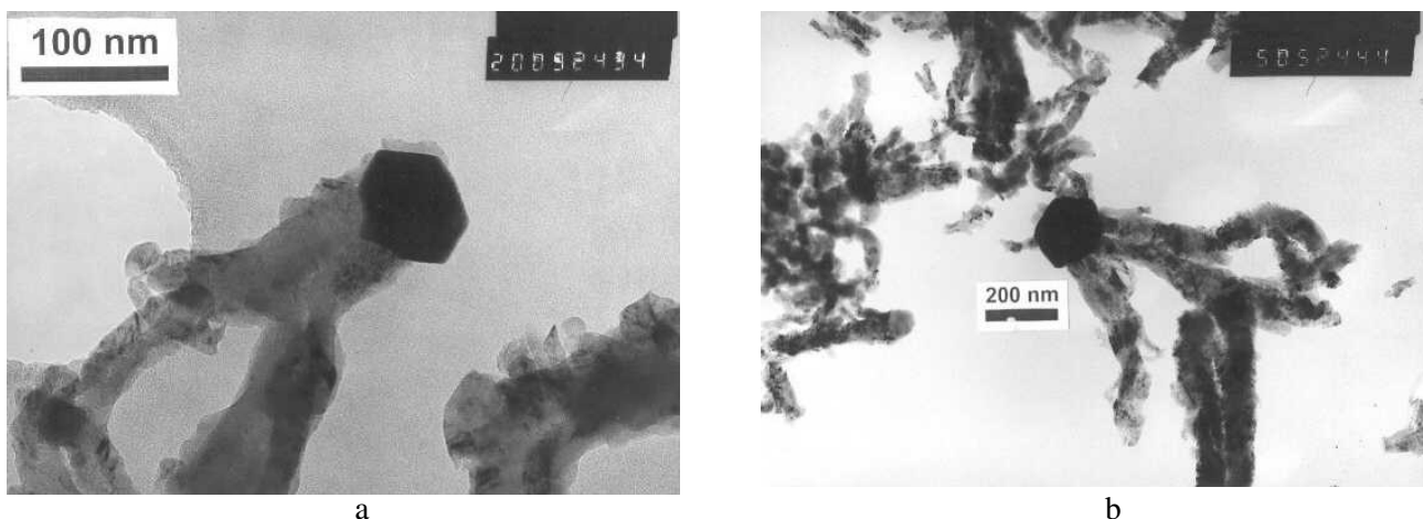
Fig. 6. TEM pictures of the samples: 82Ni8Cu (a), 75Ni15Cu (b) after 2 hours of methane decomposition at 650°C.
